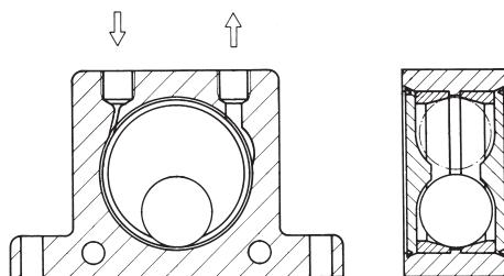
Housing made from extruded aluminium alloy
