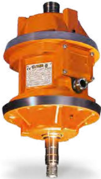
The VB series is made up of vertical vibrators with double conical flange. These vibrators are typically used in circular screens and in medium-size and large sieves. They are supplied without eccentric weights, which must be realised and mounted by the manufacturer of the vibrating machine.
